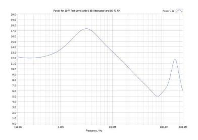
Measured amplifier power to achieve the highest level required in EN 61000-4-6 of 10 V. Measurement was carried out with 6 dB attenuator and 80% amplitude modulation.
