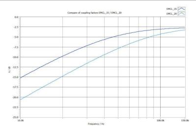
The high coupling factor of the EMCL-35 allows a test according to level 3 (10V) of IEC 61000-4-6 already at 10 kHz with the test generator CDG 6000-75\_10.
